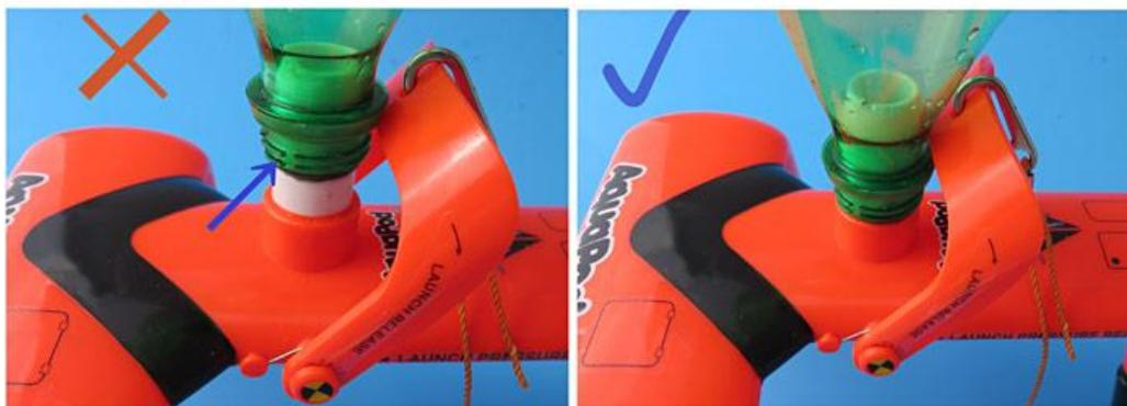
**Figure 5.** The bottle rocket needs to be pushed over the thin black ring of the launcher, as shown in the figure on the right. In the image on the left, the bottle is not pushed down far enough.
