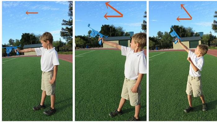
**Figure 8.** Person using the altitude finder to measure the height a rocket reaches. (Left) The rocket barely comes off the ground. (Middle) The rocket goes to medium height. (Right) The rocket goes very high. Note how the measured angles get bigger as the rocket goes higher. The angle between the arrows in red shows the measured angle, the angle between the altitude finder and the horizontal.
