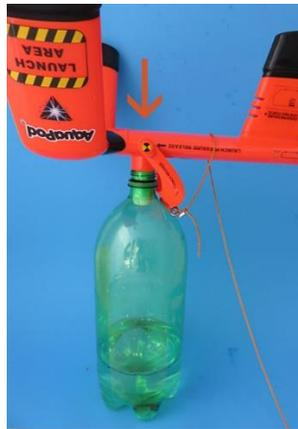
**Figure 12.** Placing the bottle rocket on the ground and pushing the launcher upside down in the bottle spout allows you to attach the rocket without spilling any water.
