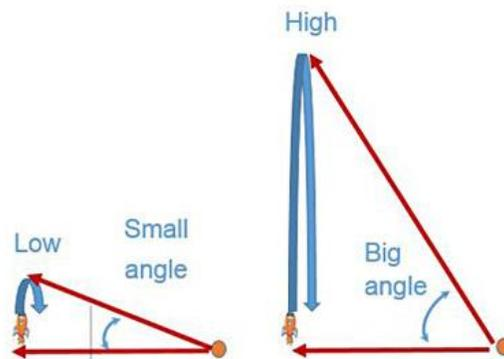
**Figure 9.** Higher points result in bigger measured angles. Note the observer is indicated by an orange dot in the figure.
