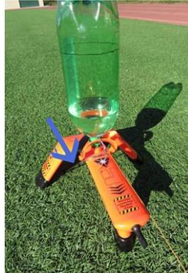
**Figure 11.** The launcher is held in place by a U peg going over the launcher and pushed into the ground.
